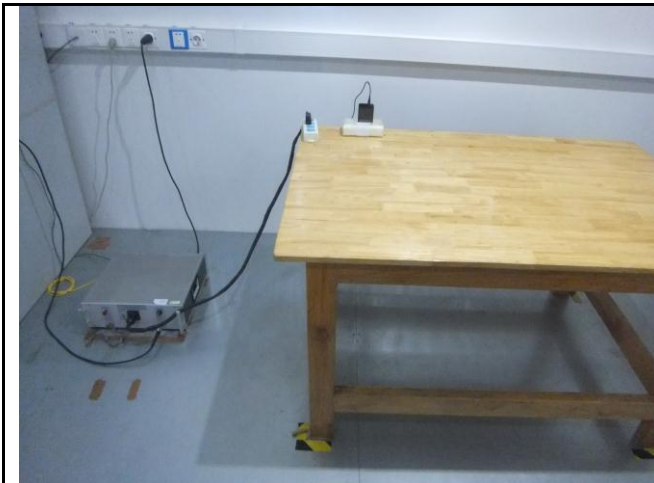
Conducted Emissions Test Setup Front View
