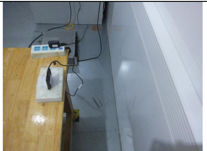
Conducted Emissions Test Setup Side View
