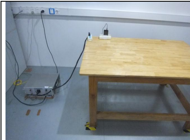
Conducted Emissions Test Setup Front View
