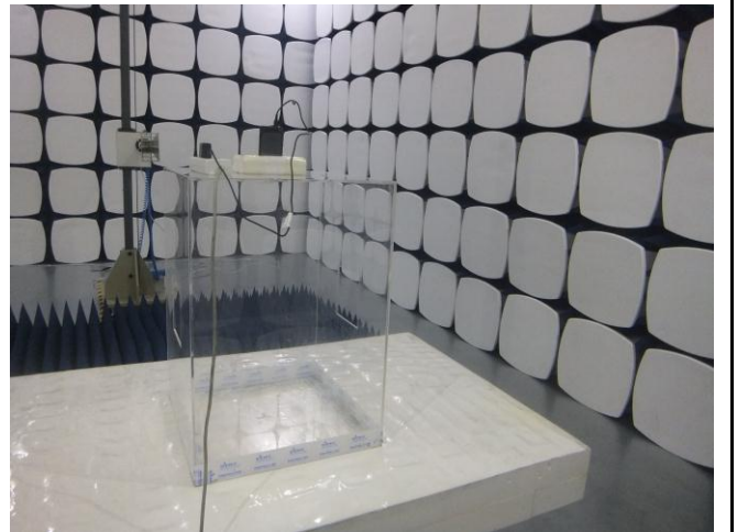
Radiated Spurious Emissions Test Setup Above 1GHz
