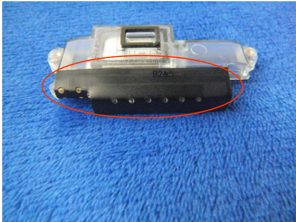
GSM/PCS/UMTS-FDD Antenna View
