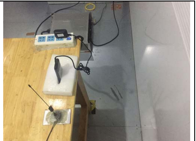
Conducted Emissions Test Setup Side View
