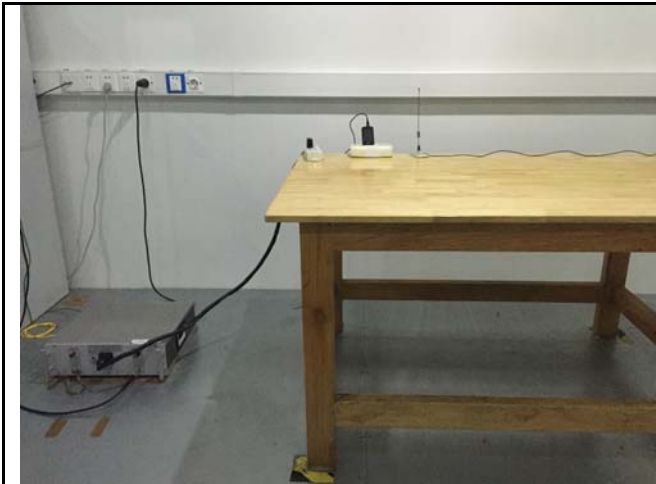
Conducted Emissions Test Setup Front View
