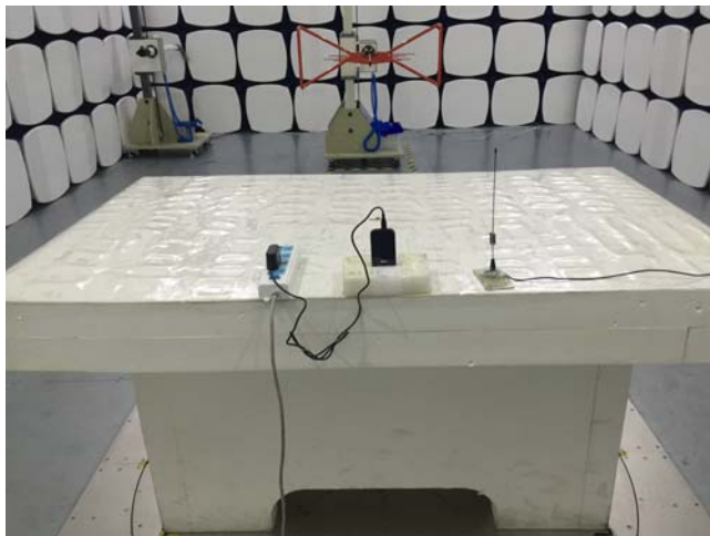
Radiated Spurious Emissions Test Setup Below 1GHz
