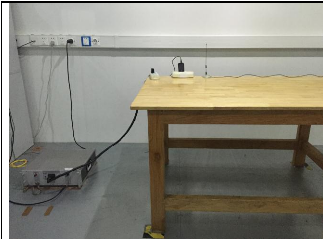
Conducted Emissions Test Setup Front View
