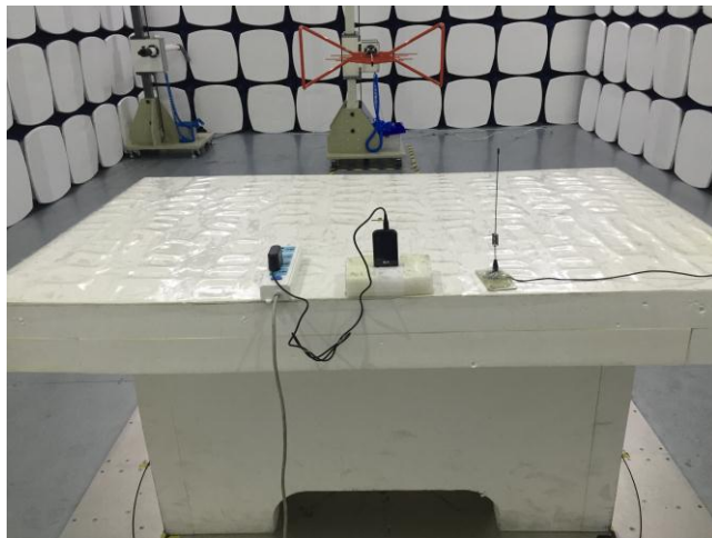
Radiated Spurious Emissions Test Setup Below 1GHz
