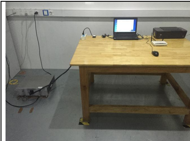
Conducted Emissions Test Setup – Front View
