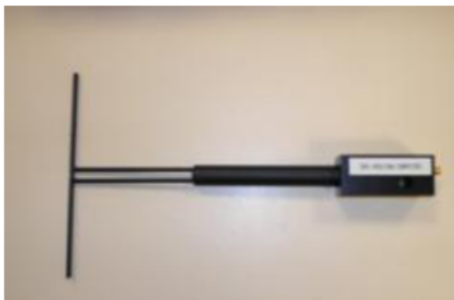
Figure 1 – Satimo COMOSAR Validation Dipole
