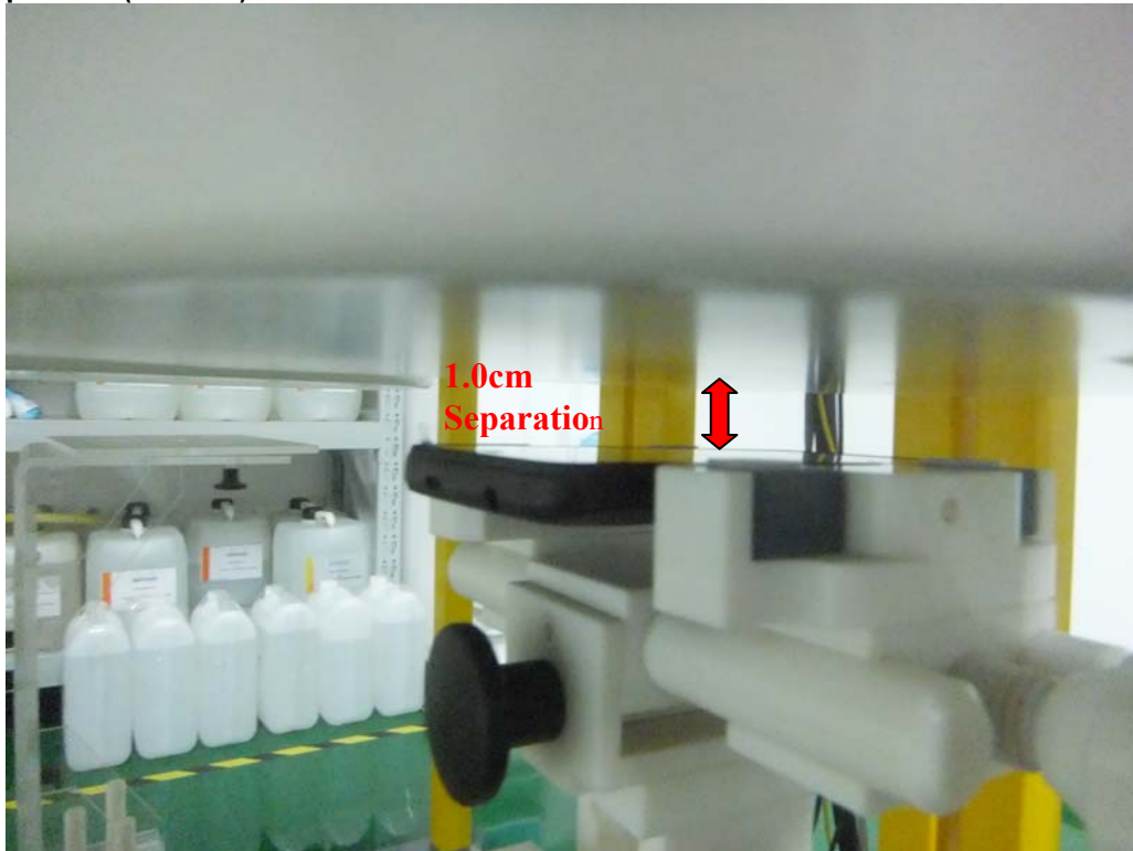
Body Setup Photo (LCD DOWN)
