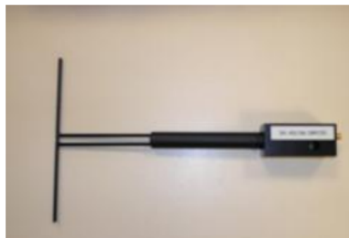
Figure 1 – Satimo COMOSAR Validation Dipole
