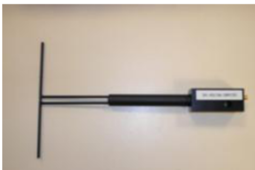
Figure 1 – Satimo COMOSAR Validation Dipole
