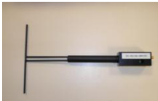
Figure 1 – Satimo COMOSAR Validation Dipole
