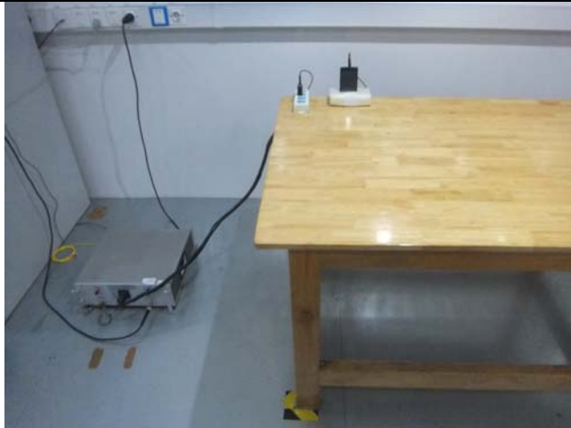
Conducted Emissions Test Setup Front View
