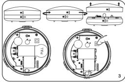
4. Attach the Water Sensor Firmly attach the water sensor to the mounted bracket. Ensure it is properly aligned and securely
