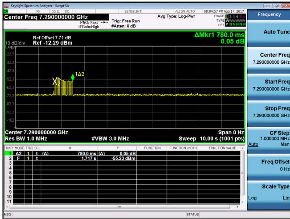
Note: The device starts transmitting and it stops transmitting in 780ms without ACK .
