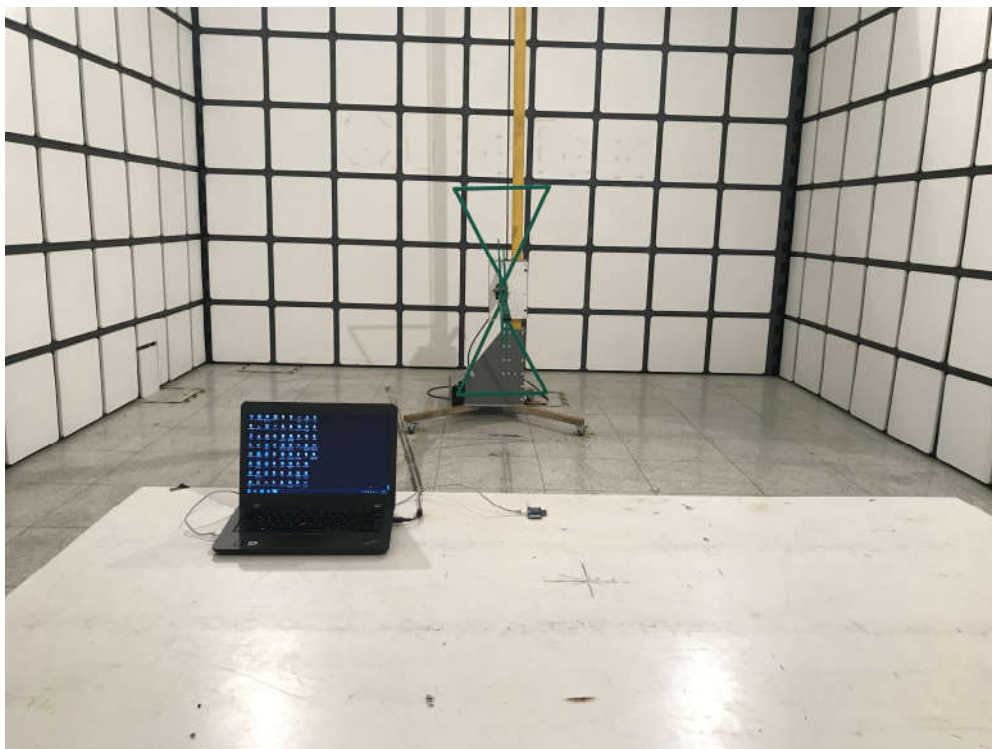
Description: Radiated Emission Test Setup for Below 1G
