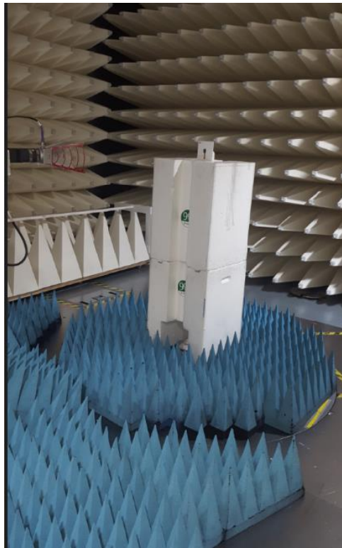
Figure B3: Radiated High range Setup 960 MHz – 18 GHz
