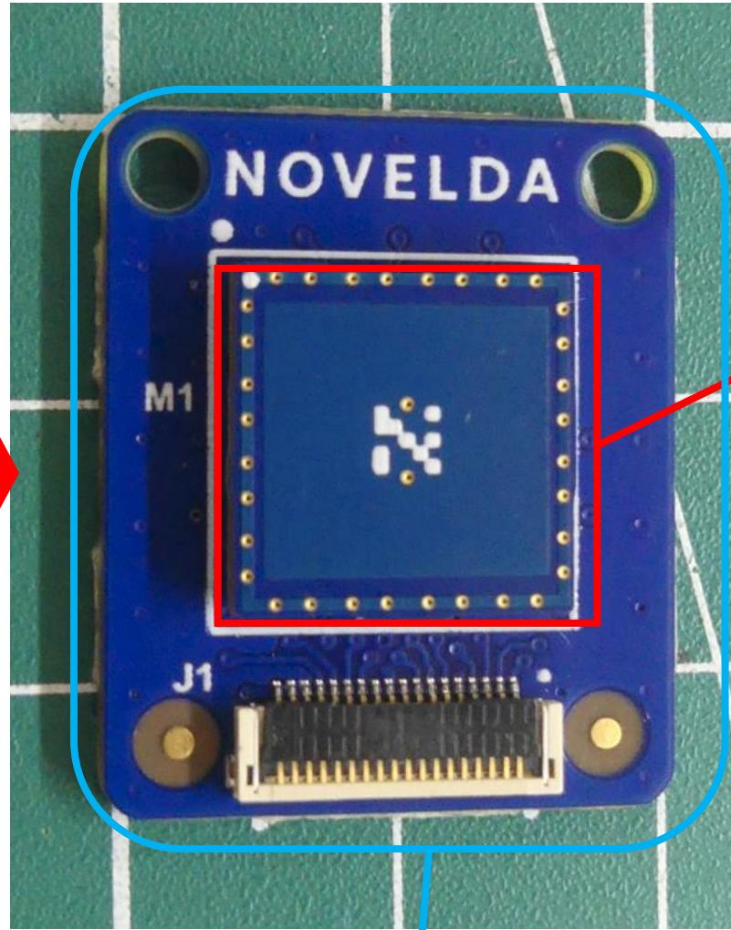
The actual module is soldered to a board with connector to control operation via the test jig
