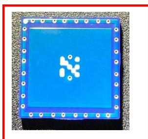
The back side of the module is the antenna.
