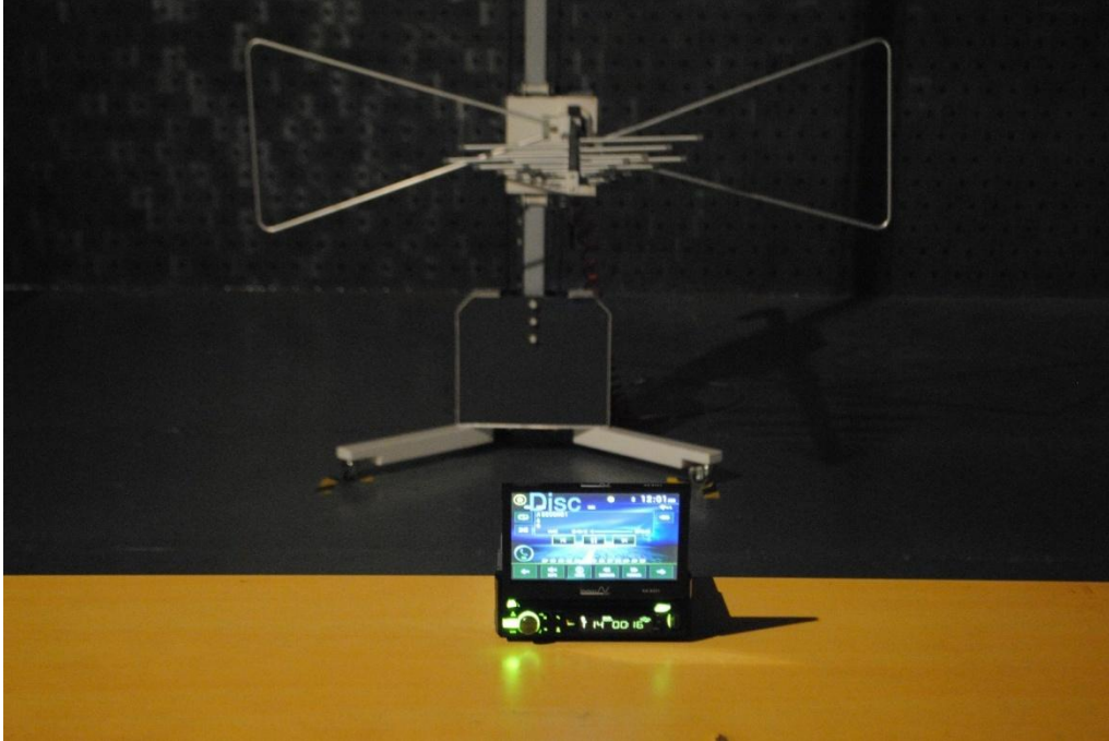
Radiated Emission test view(Frequency above 1GHz)
