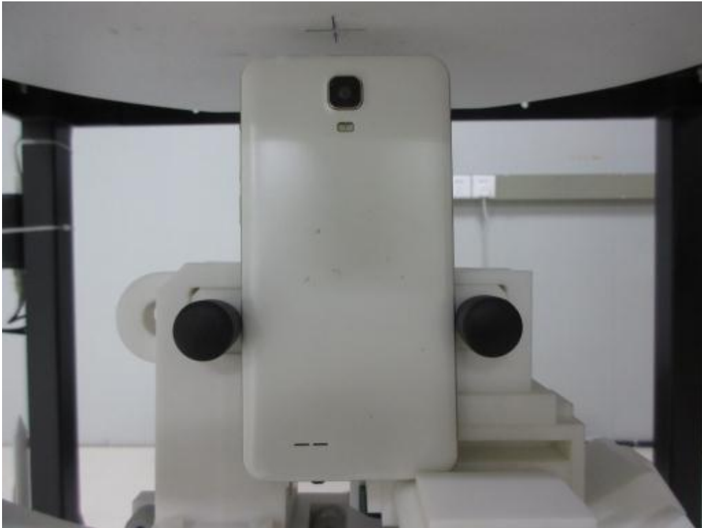
10mm body-worn Top Side Setup Photo(hotspot)
