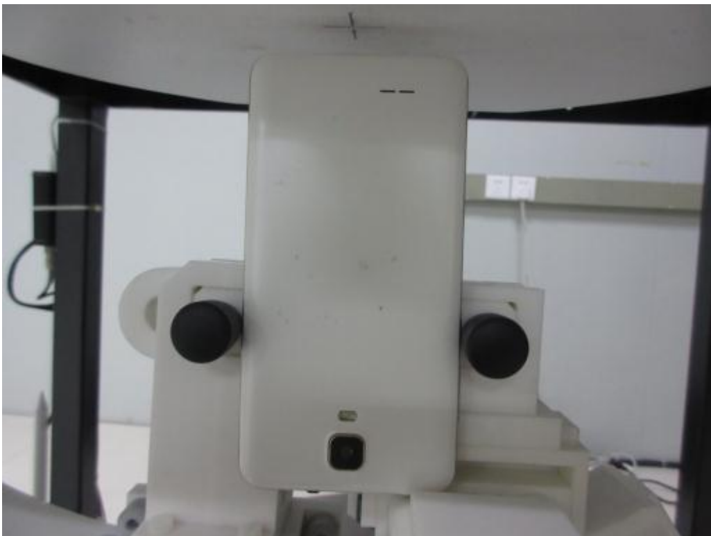
10mm body-worn Bottom Side Setup Photo(hotspot)
