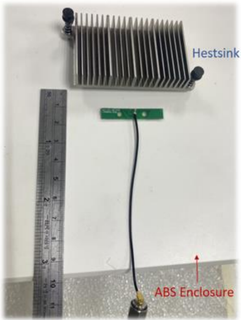
Antenna tested with ABS Antenna is 10mm away from metal
