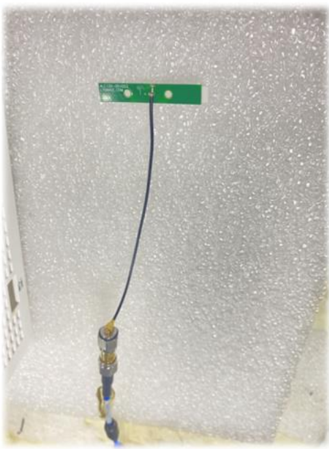
Antenna tested in free space
