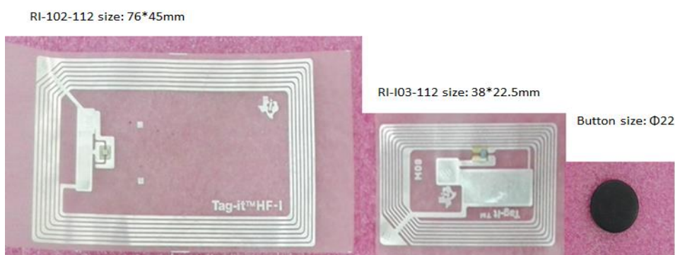
FIGURE 6.1.3 THE DIFFERENT RFID TAGS USED FOR MEASUREMENT
