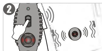
In order to avoid signal disconnection under water, please use the wireless remote controller as close as much to the back receiver of the undersuit.
