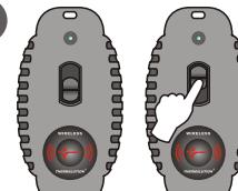
Push the button upward once to adjust between the temperature settings:
