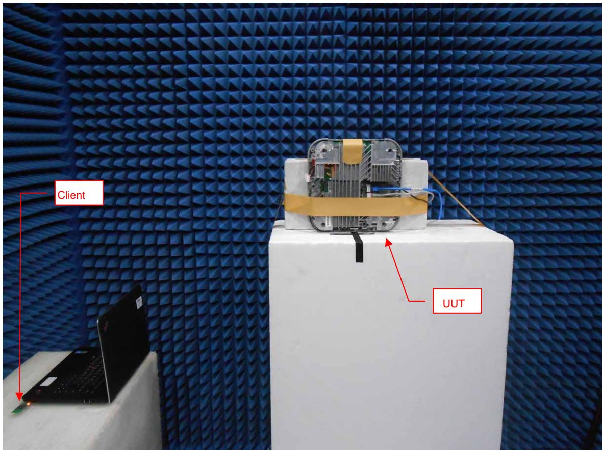
Note: Starting WiFi Module was installed in test fixture with heat sink for the test.
