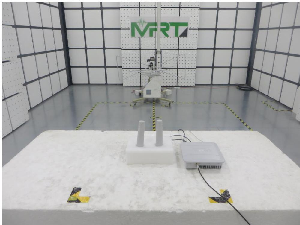
Description: Radiated Spurious Emission Test Setup for 1GHz ~ 18GHz (Omni Antenna)
