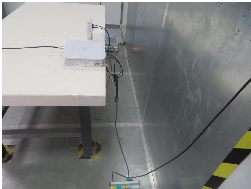
Description: Radiated Spurious Emission Test Setup for 30MHz ~ 1GHz (Directional Antenna)
