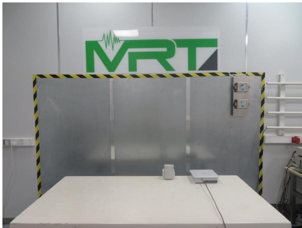
Description: Back View of Conducted Emission Test Setup (Directional Antenna)
