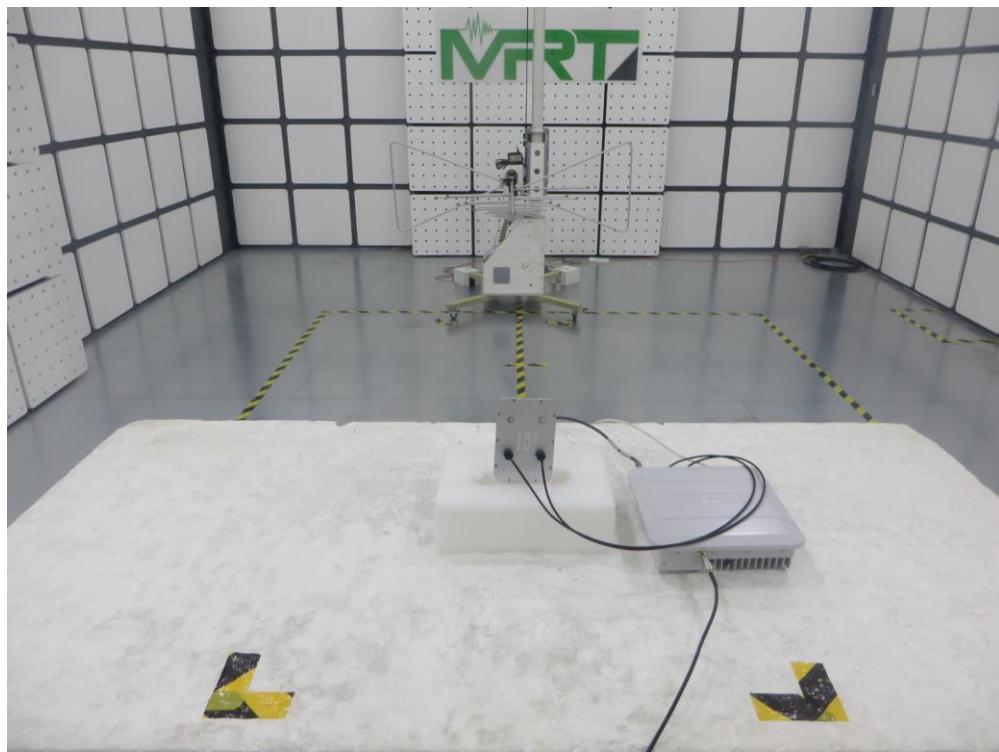
Description: Radiated Spurious Emission Test Setup for 1GHz ~ 18GHz (Directional Antenna)
