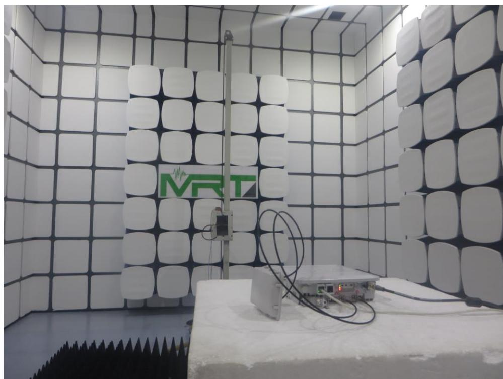
Description: Radiated Spurious Emission Test Setup for 30MHz ~ 1GHz (Omni Antenna)
