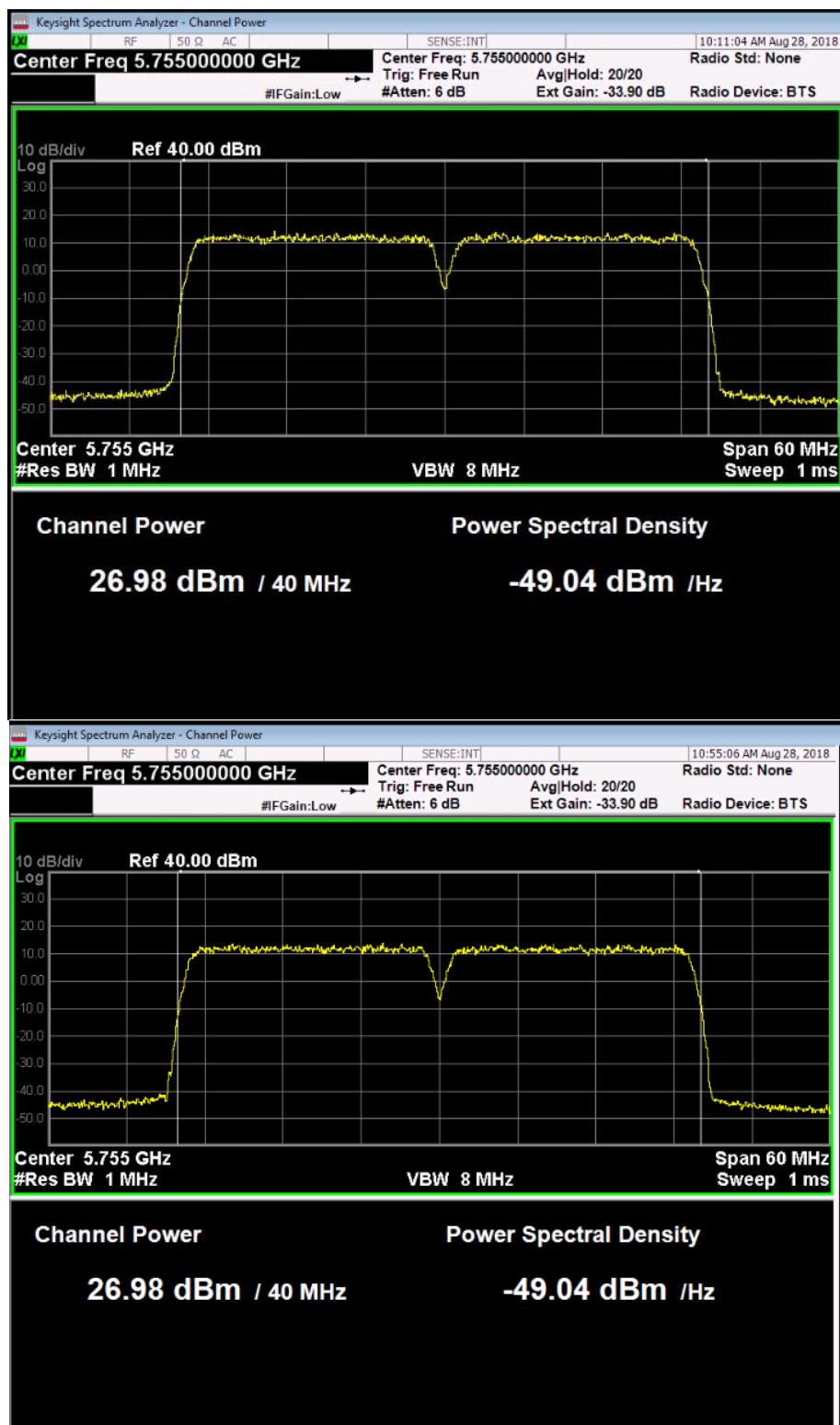
Figure 4.6.2(a) The Mean Output Power Measured for UNII-3 Q/16Q 2x20MHz Carriers at 5745MHz and 5765MHz, 27dBm, Port 1 & Port 2, for EUT with Antenna #2 (Combined Output Power 30.0 dBm).
