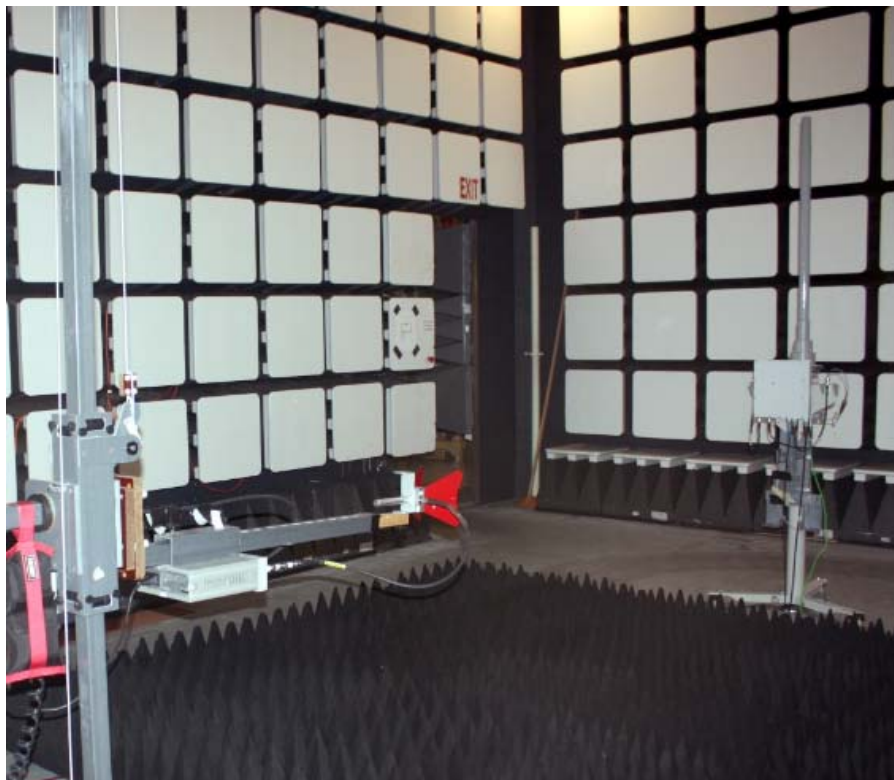
Figure 5. Setup Photo of Radiated Test
