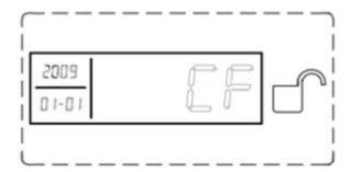
Press "\(\bigcap\)" button on remote controller or "\(\bigcap\)" button on panel and the system will be armed with BI BI tones or "DISARM" human voice. The system won't alarm for any trigger under the status of disarmed, except for emergency alarm
