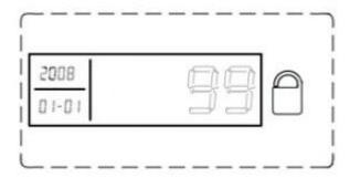
Press "♣" button on remote controller 1 time, the system will show 99 flashing on the LCD display, and also start calling/SMS with silence. But if you press "♣" button again, the siren will start at once
