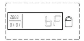
Press "\new" button on remote controller or "\overline" button on panel, the system will be home armed with BI tone and and "intelligent defenses" human voice. The system won't alarm for trigger at home arm zone under the status of home arm
