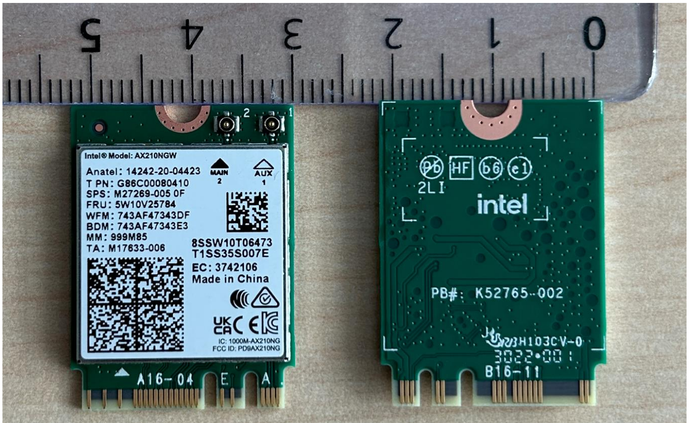
Figure 7: front- and backside of the radio module. The size of the PCB is 22 x 30 mm².
