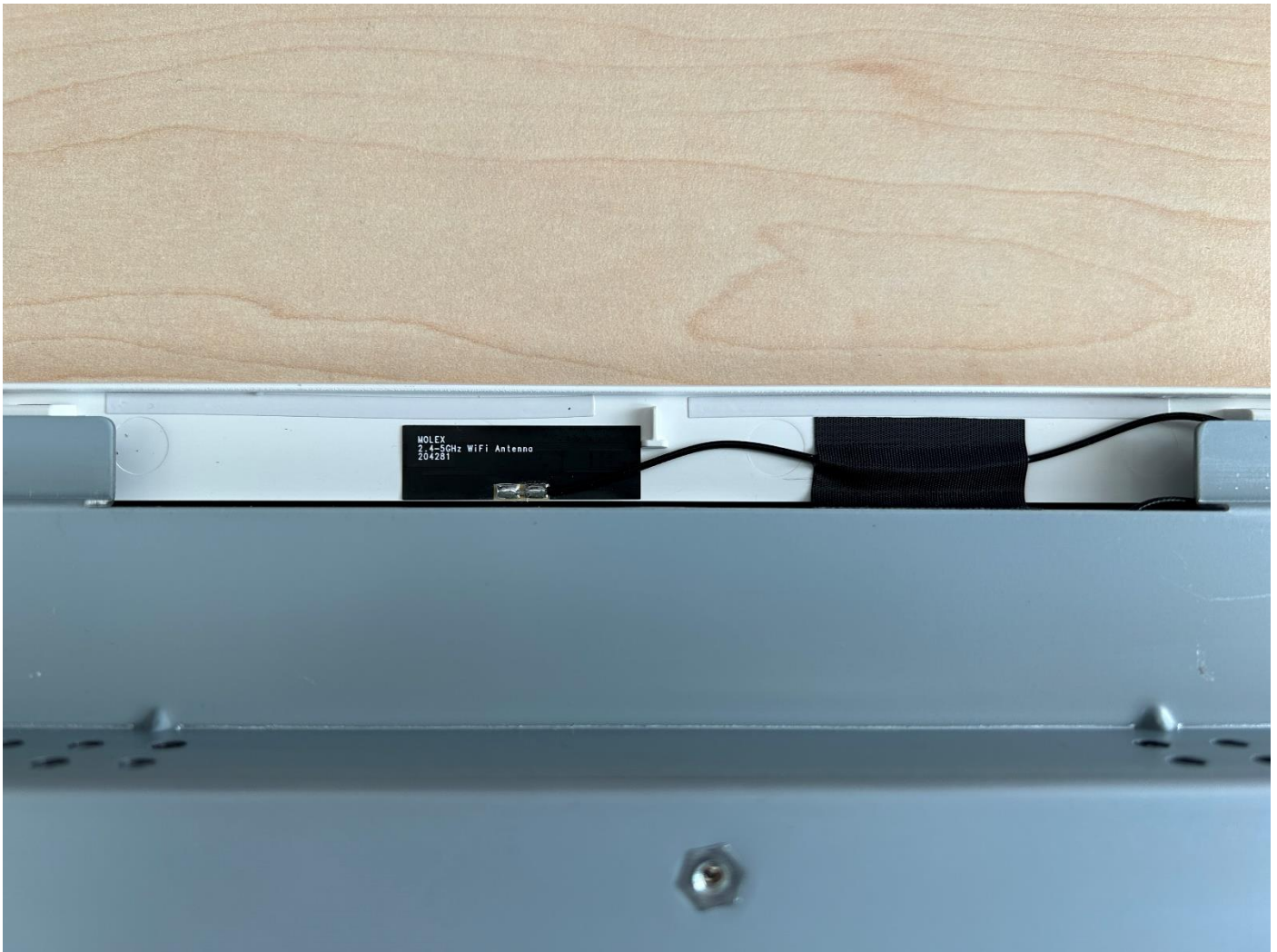
Figure 3: close-up of the antenna attached to the top of the AIO display. The size of the antenna is 35 x 11 mm².
