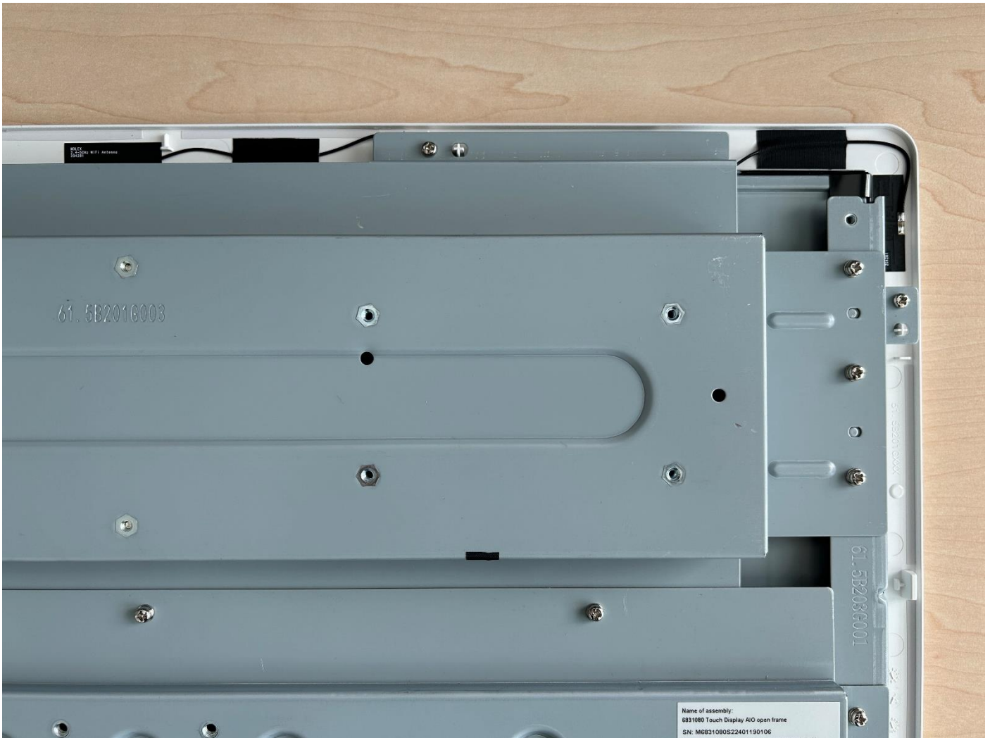
Figure 2: close-up of Figure 1. The 4 bolt holes in the middle are used to mount the single board computer. The 2 antennas are also visible on the top left (attached horizontally) and top right (attached vertically).
