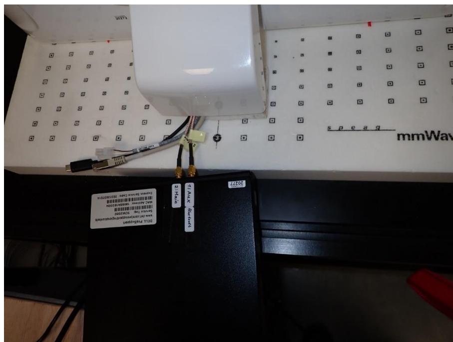
Figure D.6: DUT test set for top side.
