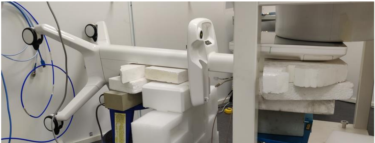
Figure 7 The spot-check test configuration with stand, front side of the device against to phantom, 0mm separation.
