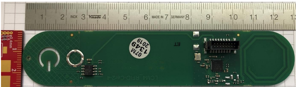
Pict. 2: RFID Transponder, component side, outer dimension 130mm x 26mm
