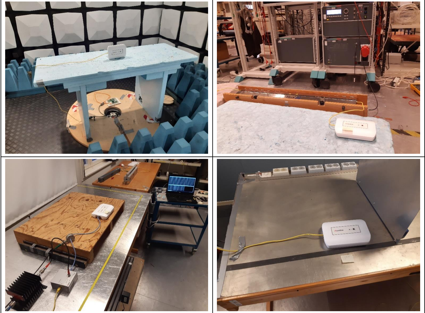
Test set-up for EMC immunity tests
