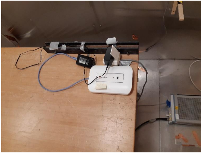
Test set-up for EMC emissions measurements
