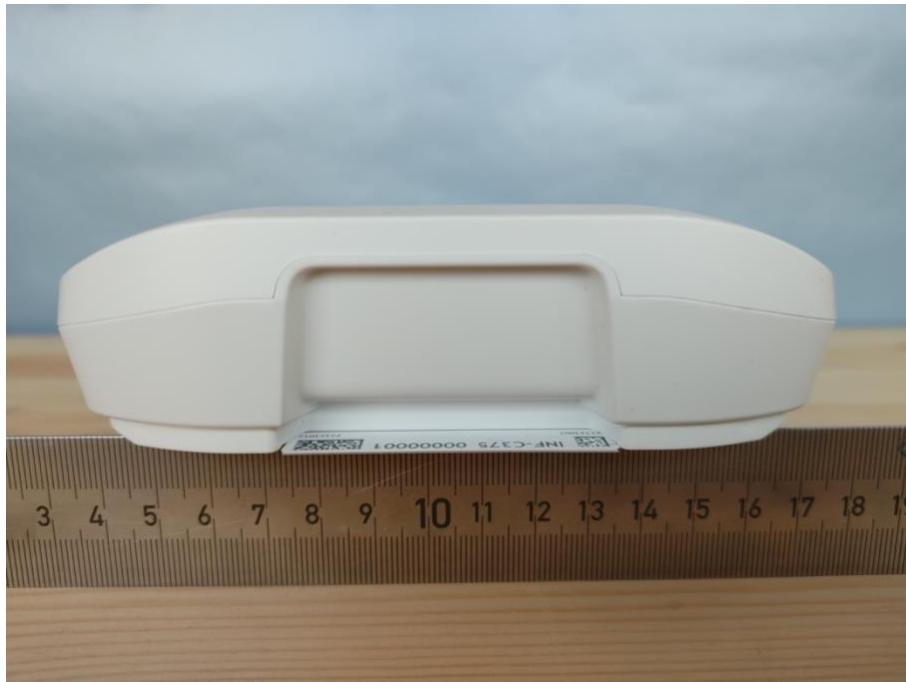
Figure 4: Photo of INF-C365 and INF-C375, showing the side with the label for the serial number. The only difference for INF-C365 is that “INF-C375” will be replaced with “INF-365” on the label.
