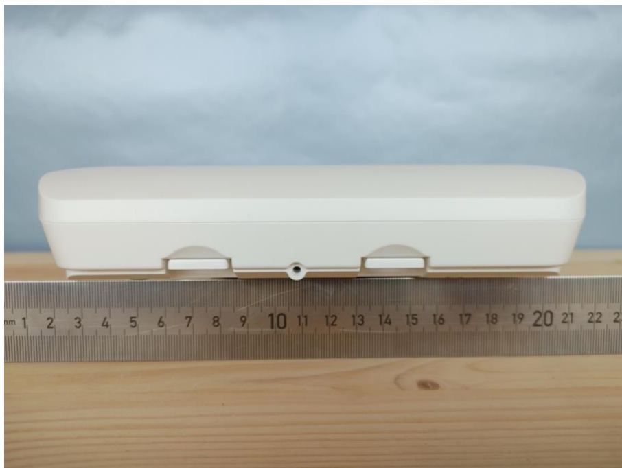
Figure 5: Photo of INF-C365 and INF-C375, showing the side with the opening mechanism.
