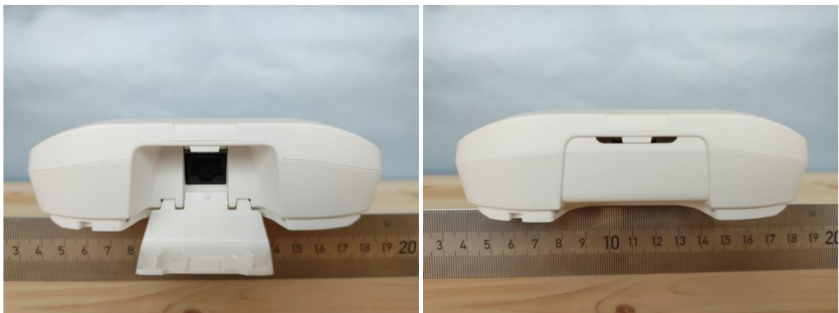
Figure 3: Photo of INF-C365 and INF-C375, showing the POE inlet uncovered (left) and covered (right), as explained in the User Manual.
