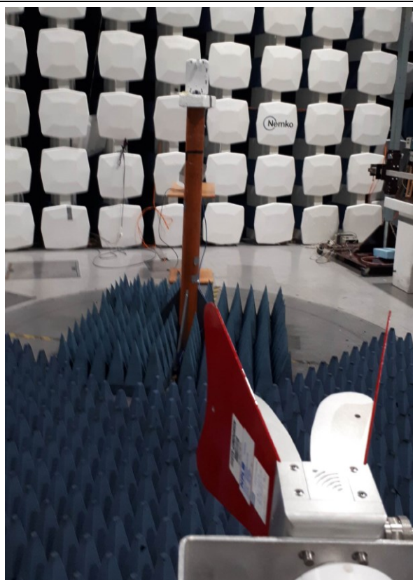
Radiated Emissions 1 – 18 GHz from antenna, device in YZ-orientation The EMC 3117PA antenna is used for spurious measurements
