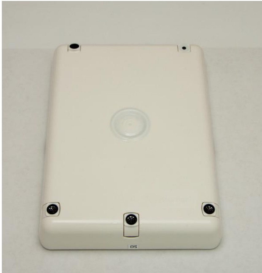
Figure 1 INF-B246-C front with one omni-directional and four directional waveguides. The unit in the picture is the INF-B246-C sample used during the FCC testing.
