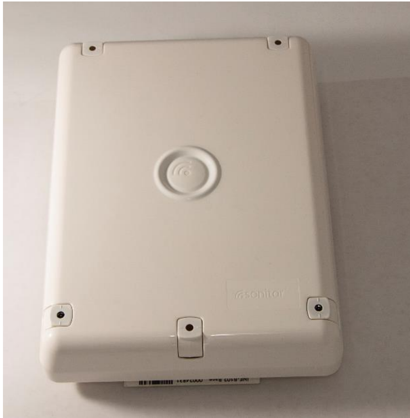
Figure 5 INF-B216 front with one omni-directional waveguide (the middle one on the lower part of the enclosure). The other four transducer housings are empty (see the Top inside pictures).
