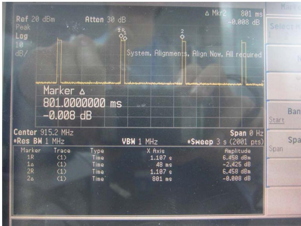
2. The Max Power (Max Tune-up Power is 18 dBm)
