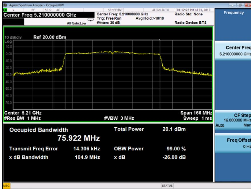
Emission Bandwidth&99% Occupied Bandwidth UNII Band II-A
