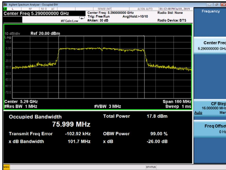
Emission Bandwidth&99% Occupied Bandwidth UNII Band II-C
