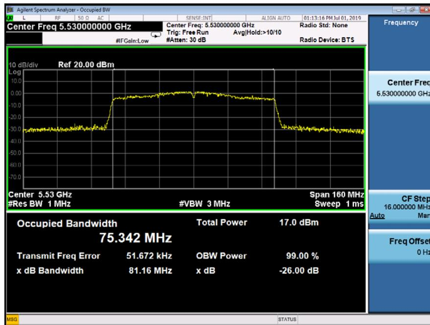
Emission Bandwidth&99% Occupied Bandwidth UNII Band II-C
