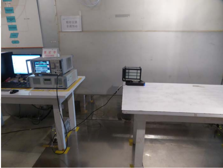
TEST SETUP OF CONDUCTED EMISSION
