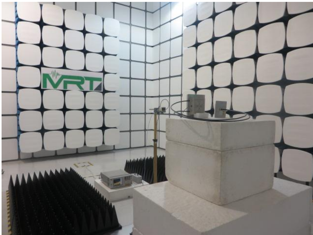
Description: Radiated Emission Test Setup for 18GHz ~ 40GHz(2.4GHz)
