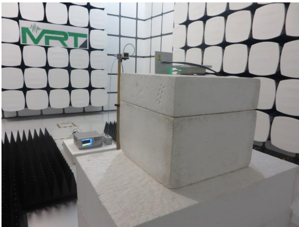
Description: Radiated Emission Test Setup for 18GHz ~ 40GHz(5.0GHz)
