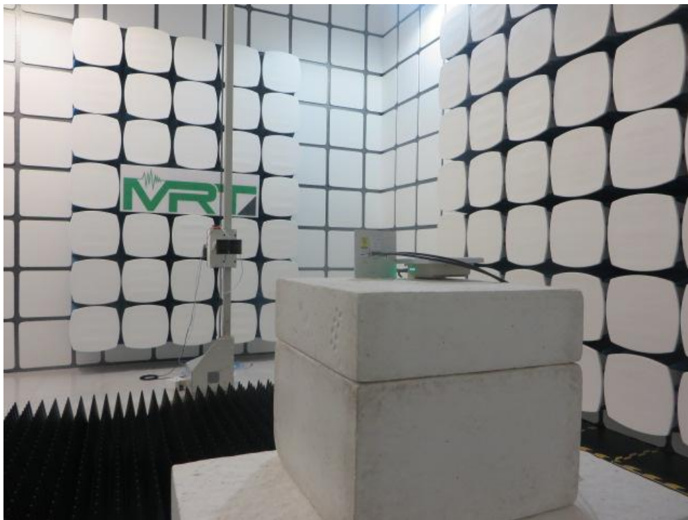
Description: Radiated Emission Test Setup for 18GHz ~ 40GHz(5.0GHz)
