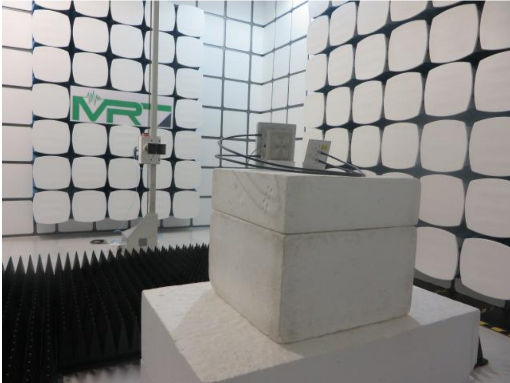
Description: Radiated Emission Test Setup for 18GHz ~ 40GHz(2.4GHz)
