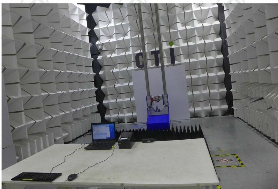
Radiated spurious emission Test Setup-3(Above 1GHz)
