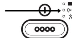
During power-up, if all LEDs are blue the sensor has not powered up correctly.
