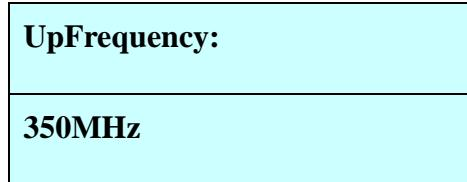
The transmitter upper frequency could be adjusted by UP or DOWN with step 1MHz and range 100-3000MHz.
