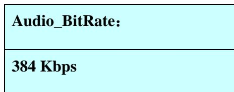
It shows the current audio input bitrate, which is only readable under AUTO mode, adjustable by UP and DOWN under Manual Mode. The single-track audio bitrate range: 32kbps, 48kbps, 56kbps, 64kbps, 80kbps, 96kbps, 112kbps, 128kbps, 160kbps and 192kbps; dual track bitrate range: 64kbps, 96kbps, 112kbps, 128kbps, 160kbps, 192kbps, 224kbps, 256kbps, 320kbps and 384kbps.
