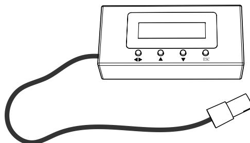
LCD modules are combined with LCD display and three buttons. From the left to right there are menu button **◀▶**, up key **▲**, down key **▼** and cancel button **ESC**, 4-core plug interface.
