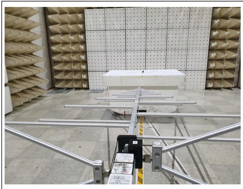
**3. Photo of Radiated Spurious Emission Test (Above 1 GHz)**
