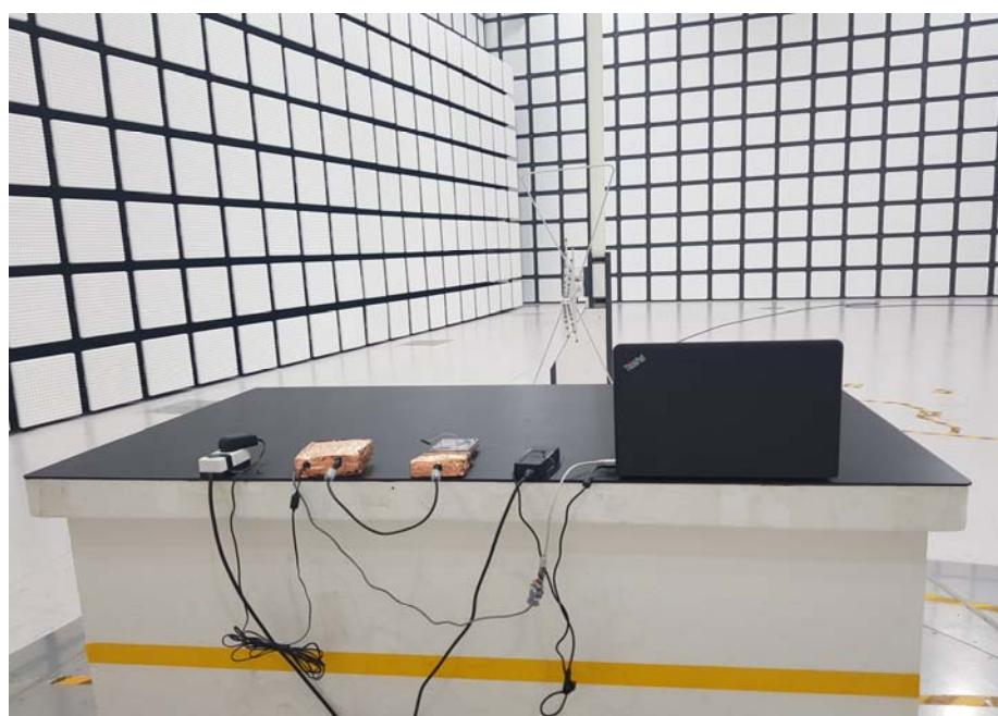
3. Radiated Emission setup photo (above 1 GHz)
