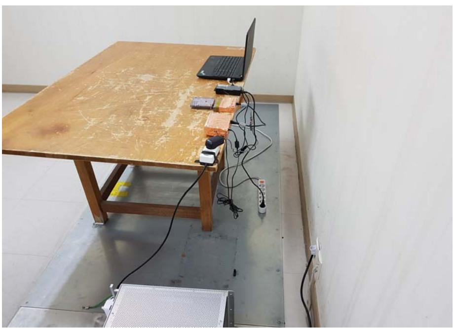
2. Radiated Emission setup photo (below 1000 MHz)
