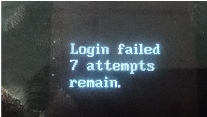
If retry count of 10 is already tried, then a message "ORWL LOCKED !!!" will be displayed and the device needs to be sent to factory for unlocking it.
