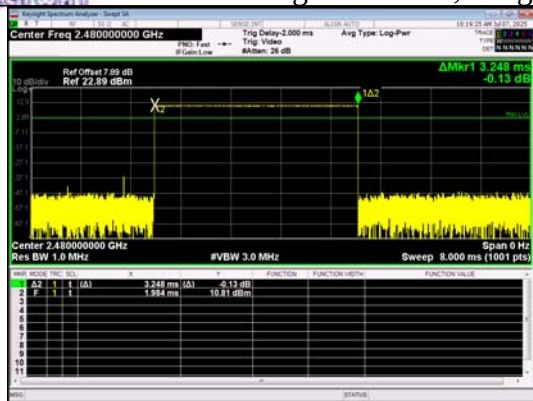
Pulse Width GFSK DH5
