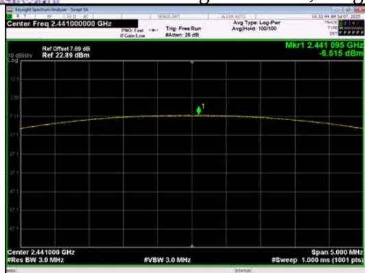
Peak Output Power \pi/4 DQPSK_Channel 39
