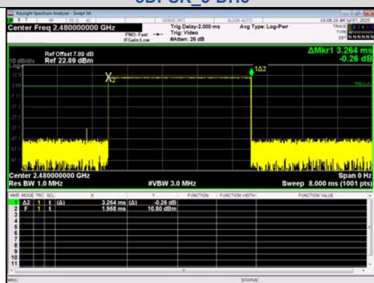
Pulse Width 8DPSK_3-DH5
