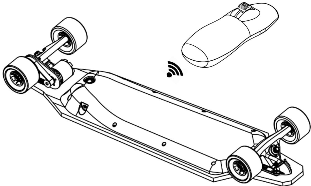
Every Falcon Cruiser is connected with its controller through a unique radio frequency. You will hear beep sounds after turning on the Falcon Cruise and its controller. The matching is completed when the beep finished.
