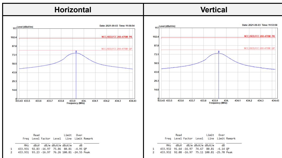
**Below 1G (30 MHz-1 GHz) test the output power worst mode:**
