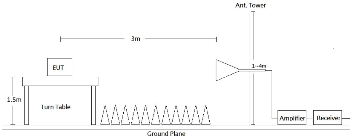
Radiated emission tests were performed in the 3 meters chamber test site, using the setup accordance with the ANSI C63.10-2013. The specification used was the FCC 15.209, FCC 15.205, and FCC 15.231 limits.
