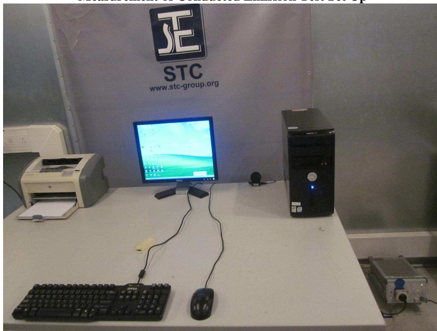
Measurement of Conducted Emission Test Set Up
