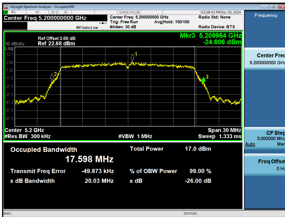
-26dB Bandwidth NVNT n20 5200MHz Ant2
