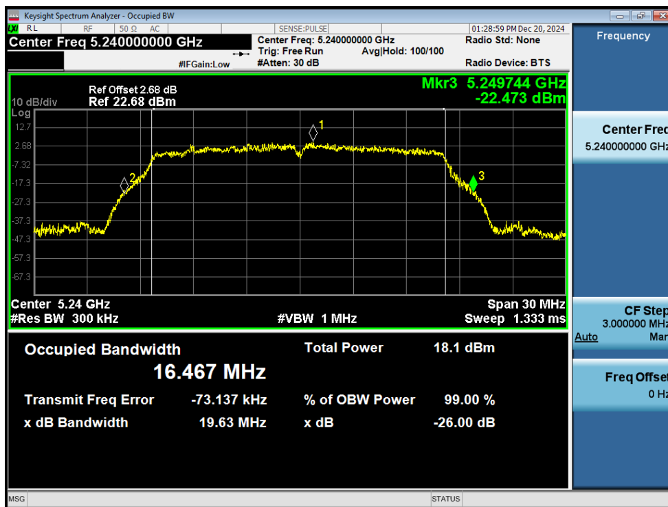
-26dB Bandwidth NVNT a 5240MHz Ant1
