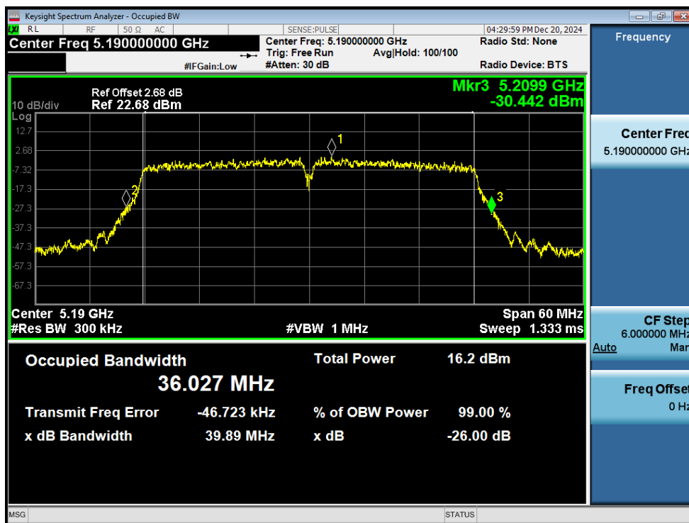
-26dB Bandwidth NVNT ac40 5190MHz Ant2
