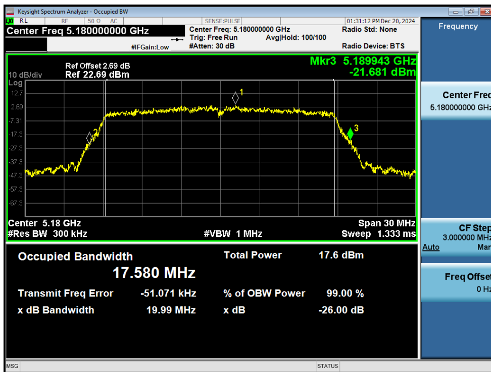
-26dB Bandwidth NVNT n20 5180MHz Ant1
