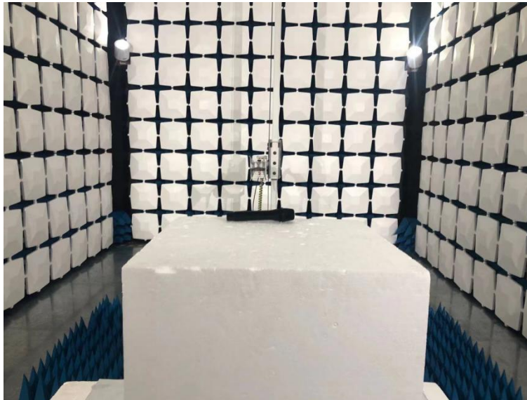
Below 1GHz for radiated emission test setup
