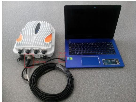
3.Insert the power connector into the powerinlet on the interface, and then plug the power adapter into an electrical socket.
