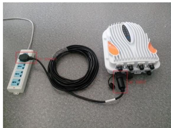
4.Insert the connector of antenna into one of the four antenna ports of the XDUR-840 UHF RFID Reader. You can connect at most four antennae at the same time.
