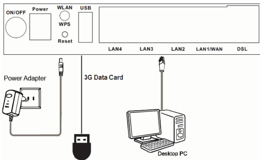
**Note:** SIM card is properly inserted & ISP Service is activated before inserting USB mobem into the router
